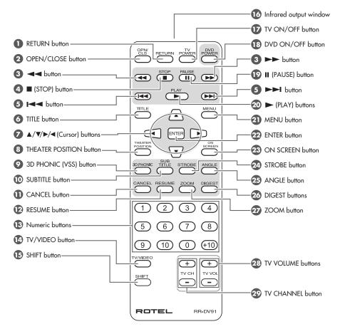
**Infrared signal-emitting window** Point this window toward the remote sensor on the front panel when pressing buttons.
